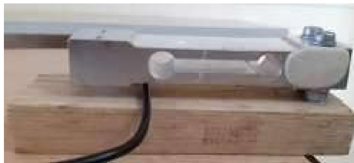
Fig. 3 Load Cell mounting
