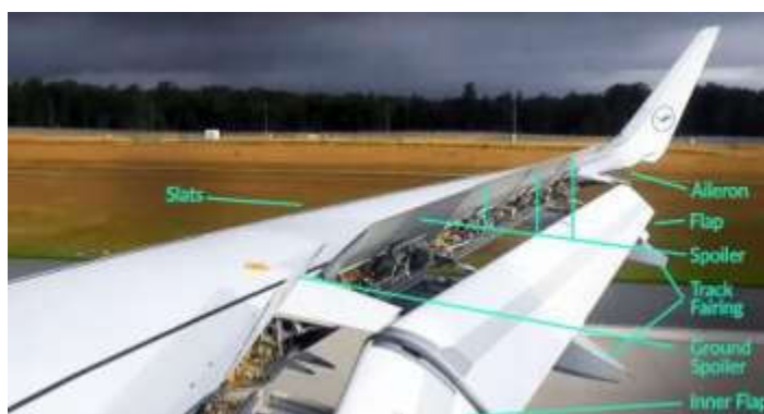
Fig 5: Structures associated with the wings
