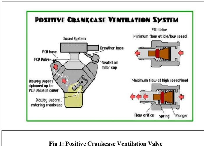
Fig 1: Positive Crankcase Ventilation Valve
