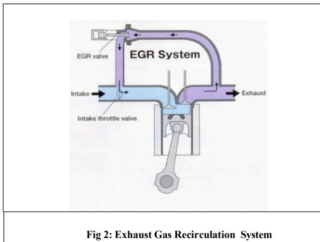
Fig 2: Exhaust Gas Recirculation System
