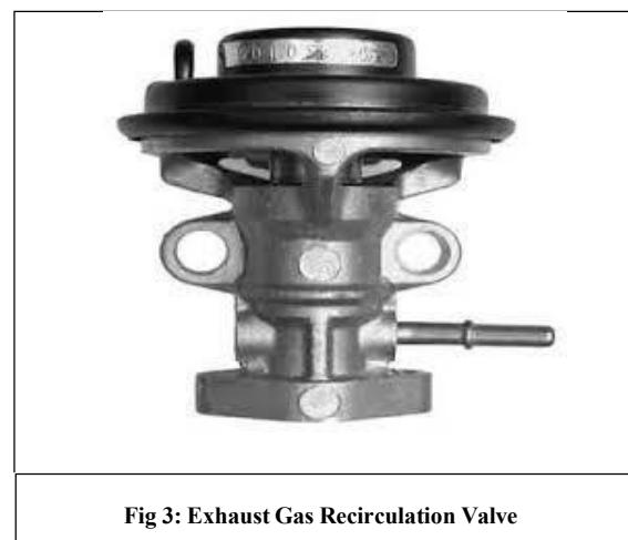
The purpose of the exhaust gas recirculation valve (EGR) is to meter a small amount of exhaust gas into the intake system; this dilutes the air/fuel mixture so as to lower the combustion chamber temperature. Excessive combustion chamber temperature creates oxides of nitrogen, which is a major pollutant. While the EGR valve is the most effective method of controlling oxides of nitrogen, in its very design it adversely affects engine performance.
