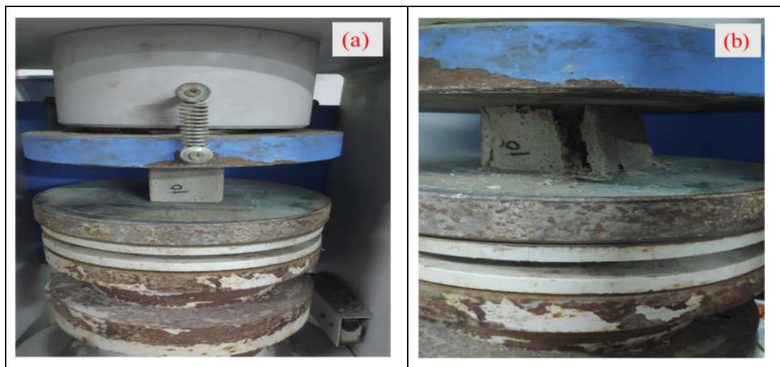
Fig. 4. Compressive strength testing: (a) specimen placement in the loading frame; (b) typical failure mode of the geopolymer mortar cube after testing.
