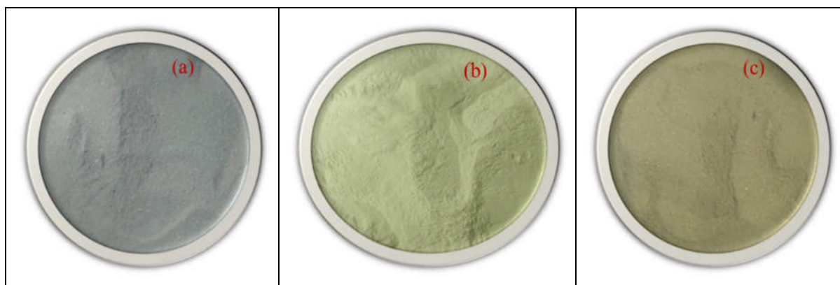
Fig. 1. Precursor materials: (a) Fly ash; (b) GGBS; (c) Tannery sludge.
