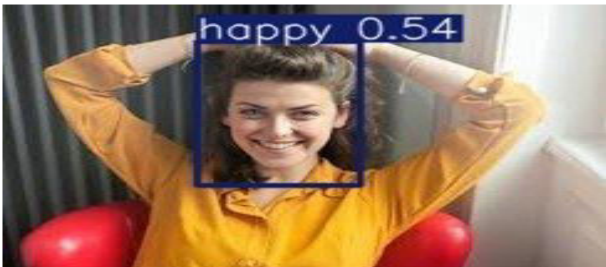
Fig. 7. Sample emotion recognition output from the SurveilAI Emotion UI identifying a happy facial expression with confidence score 0.54, with the bounding box enclosing the detected face region.
