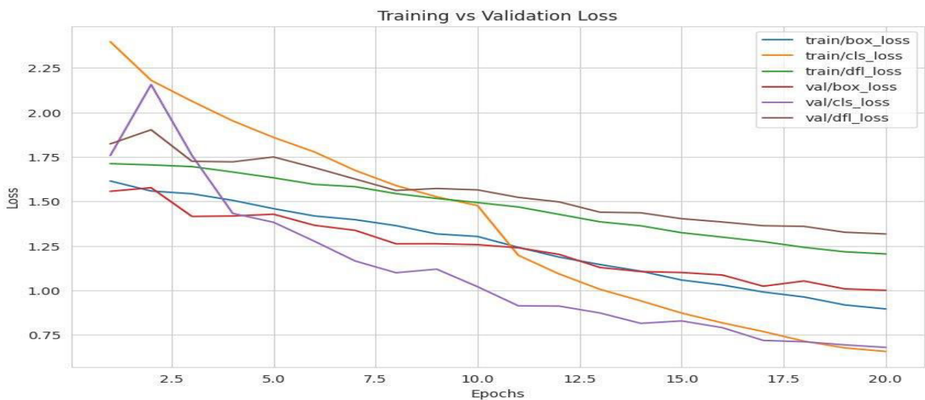
Fig. 2. Training versus validation loss curves across 20 epochs for the YOLOv8s weapon detection model, showing box loss, classification loss, and distribution focal loss for both training and validation partitions.
